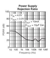
**Power Supply** Rejection Ratio vs. Voltage Drop
